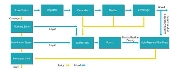
The large grains from Shale Shaker produces solids and liquid mud after flushing and dehydration. This liquid in addition with other liquid from the Desander, Desilter and the Centrifuge undergo Destabilization dozing, and separate through the filter press. The resultant liquid returns to the Mud Circulatory System, where the solids are treated safely together.
